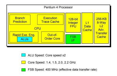
Figure 3-1 illustrates the internal architecture of the Pentium 4 processor.
